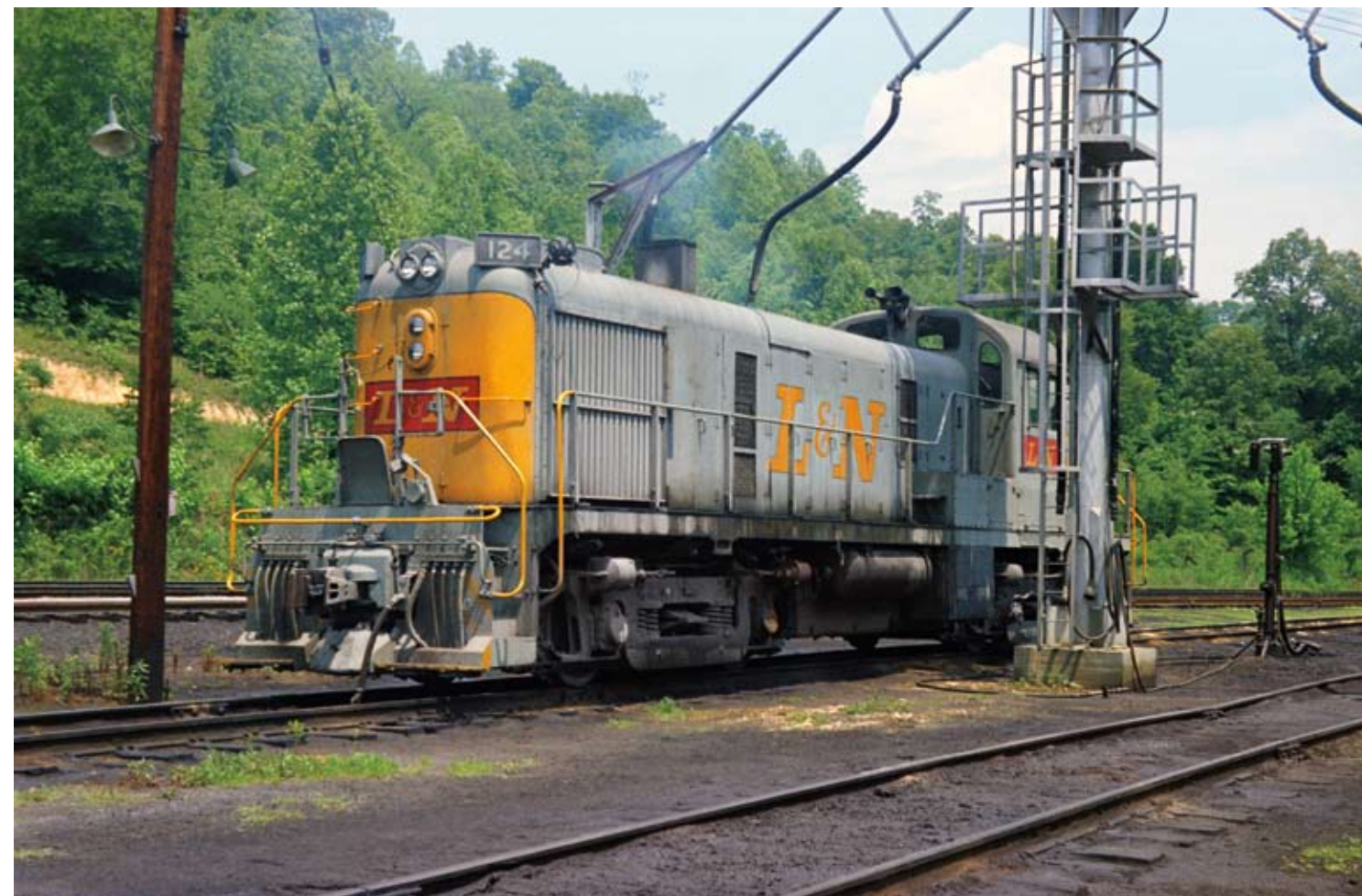
Above: The 107 members of L&N’s Alco RS-3 fleet wore the gray and yellow scheme quite well. During a break between assignments at Loyall, Kentucky, in the summer of 1965, engine 124 of this group idles quietly at the sanding and fueling area. In an hour, a crew will come calling to use the 124 on the afternoon Loyall-Varilla mine run.
